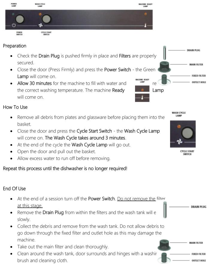
• Once cleaned replace the Drain Plug and Filters for next users.
