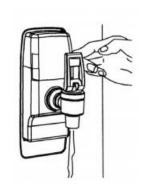
• For filling larger vessels, such as tea or coffee pots, **rotate the lever**180 degrees and pull until it locks into a horizontal position. This allows the vessel to be filled without holding your hand where it may be affected by steam. Boiling water will flow until the lever is returned to its normal vertical position.
